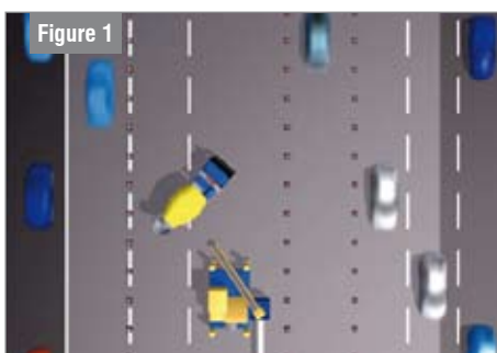
Figure 1 Typical configuration of paver and concrete supply chain
