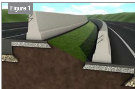
Figure 1 Dual barrier to accommodate level differences
